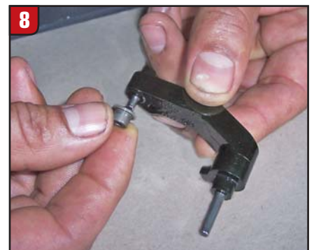
When you remove the spring tension from the detent and remove it from the selector shaft, be careful not to lose the small wheel in it, as it can fall off easily.
