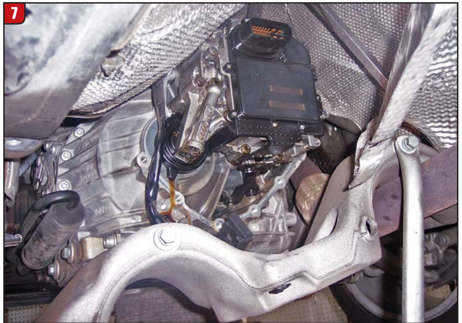
The TCM is fastened to the valve body with three bolts.
