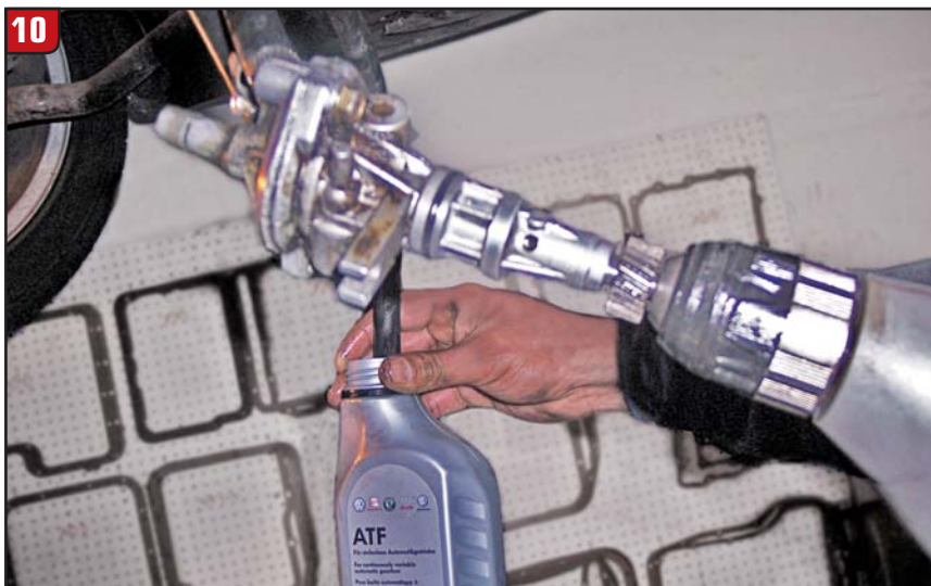
9 Checking for metal particles on the selector-shaft magnetic gate
